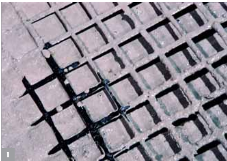
1 The C-grid replaced conventional steel reinforcement to eliminate durability problems associated with reinforcement corrosion
