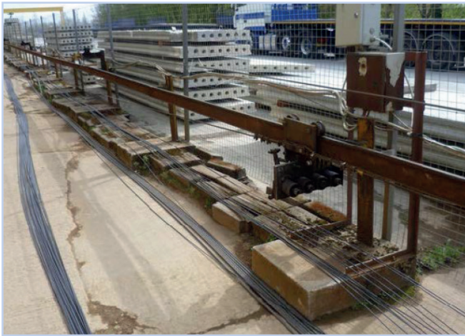
Figure 5.4 Rabbit mechanism on raised track for pulling pre-determined lengths of wire/strand.
