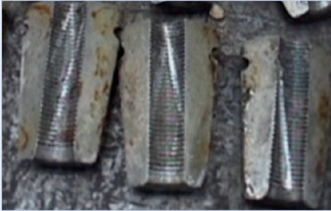
Figure 6.4 Wedges with evidence of slippage.
