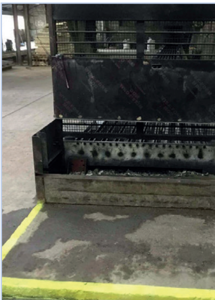
Figure 7.18 Interlocking end guards, preventing stressing until guards are lowered and fixed.
