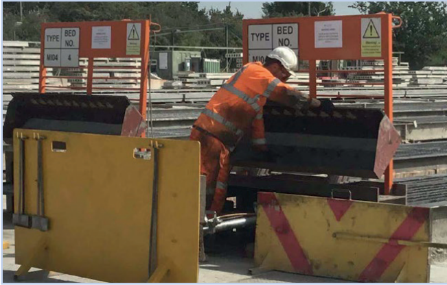
Figure 7.20 Sliding guard covering stressed wires.
