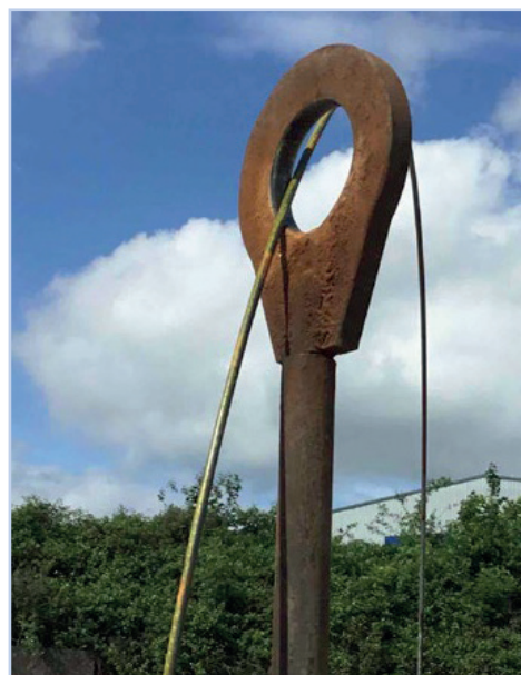
Figure 4.17 Rotating eye reducing manual handling and tangles during wire pulling.
