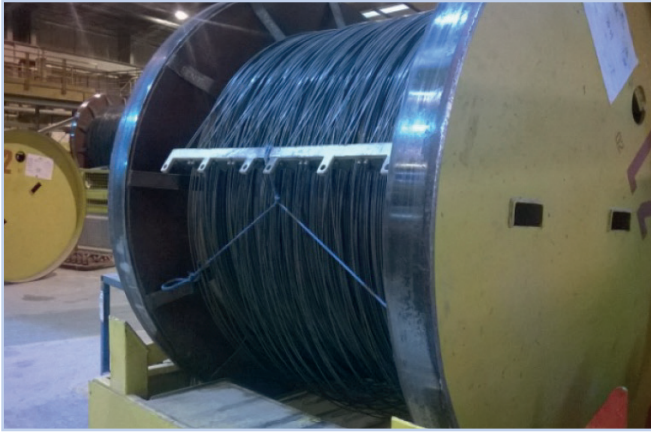
Figure 6.16 Example of completed coil ready to be moved to the bed.
