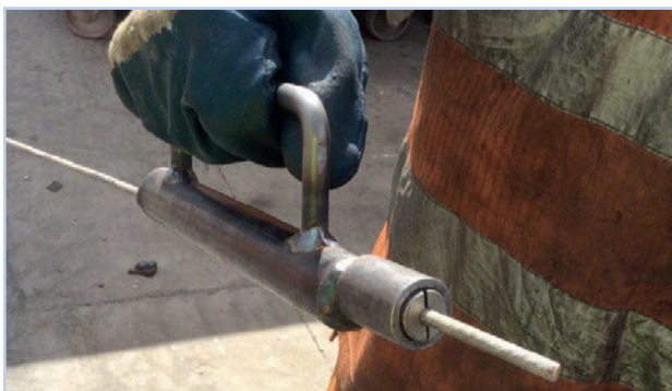
Figure 5.3 Example of tool to allow free rotation of wire when hand pulling.
