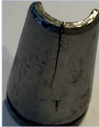
Figure 6.5 Evidence of cracked wedges.
