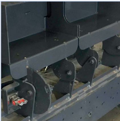
Figure 7.18 Interlocking end guards, preventing stressing until guards are lowered and fixed.
