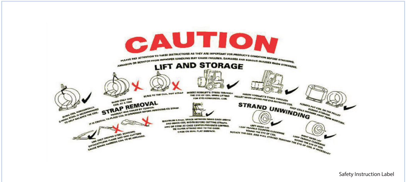
Figure 4.8 Label attached to strand as a reminder of safe handling.
