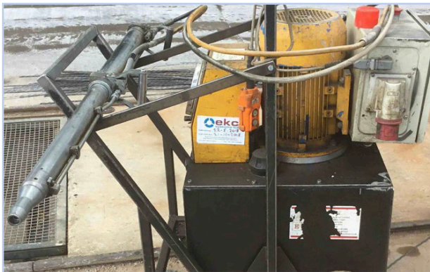
Figure 3.1 Single wire/strand stressing with a jack.
