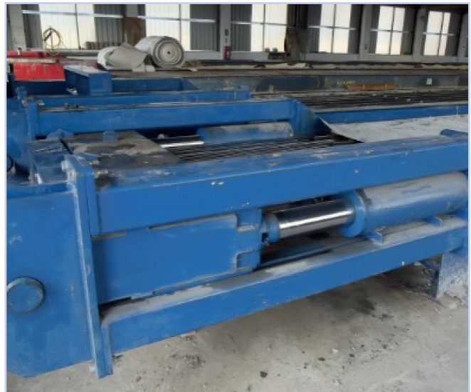
Figure 7.3 Multi-stressing mould in tensioned position.
