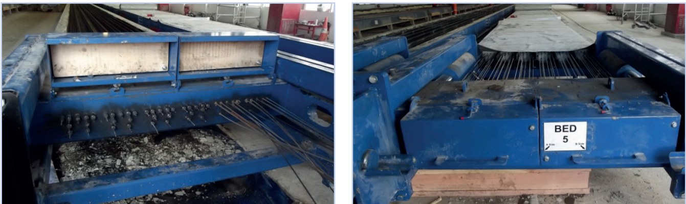
Figure 7.15 Stressing end of a wet-cast T-beam. Left: Guard raised showing timber insert used to absorb impact. Right: Guard lowered to contain all prestressed wires/strands.
