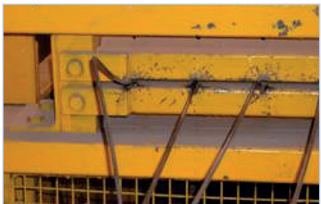
Figure 4.21 Wire/strand kinked on stressing bed.
