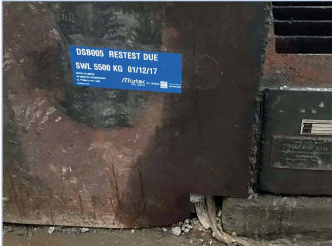
Figure 3.6 SWL and plate added to an old bed following independent verification.
