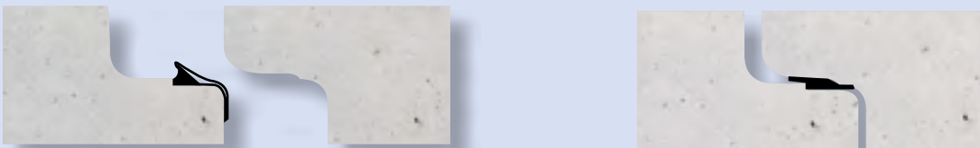
Fig. B3. Pre-lubricated Sliding Ring
