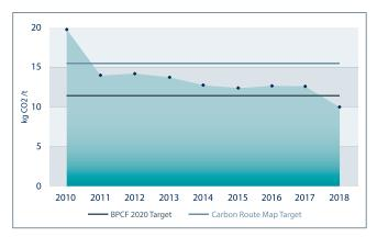
Precast factory  $CO_2$  emissions (2010-2018) against British Precast 2020 and Green Construction Board (GCB) Carbon Routemap targets.
